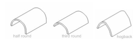
The Ridge is to be covered with either Half Round, Hogsback or mono ridge. The ridge tiles are to be edge bedded with a solid bed at butt joints. Solid bed end ridge tiles and filled with dentil slips.
